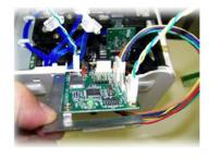
Note: Clean the plastic surface before attaching controller bracket to the base of the printer.
