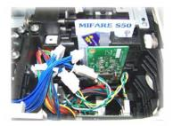
Flash the printer with Mifare card positioning firmware (PR-C101Rf\_KG-Mifare.npr) using the download utility in the properties of the driver listed under the utility tab.
